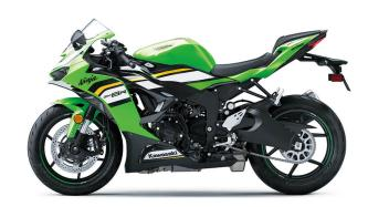
Dual semi-floating 310mm discs with dual radialmounted, monobloc, opposed 4-piston caliper,
